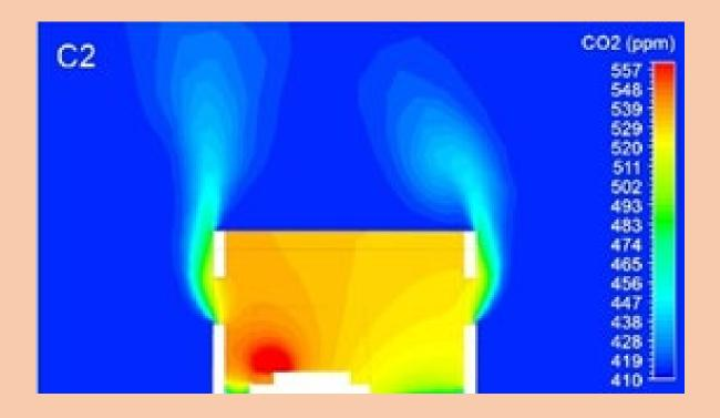
Showing carbon dioxide movement in a Gambia house with screened windows
